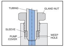
Typical Coned and Threaded port connection
