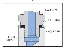
Typical port connection with British Standard Pipe (Parallel) fitting with shoulder
